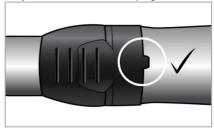
Switch the motor off after use. The black coupling can then be retracted and the attachment will come loose from the motor. To do this, hold the motor with your right hand and the attachment with your left hand. Now push the black motor coupling forward with your right index finger and thumb. The coupling will come loose.
