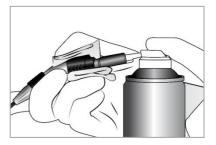
When oiling minimally invasive attachments, make sure that the minimally invasive attachment shafts (REF: VMN-T) and base unit (REF: VMN-C2) are assembled together.
