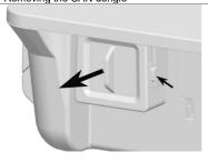
Press the locking tab on the side and remove the CAN dongle.
